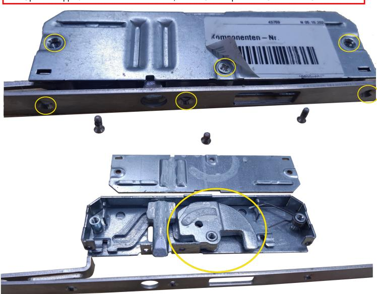
Remove the lid and remove the hook.
